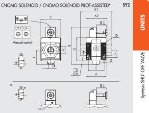
N.B.: Before assembling other Syntesi elements after the V3V, remember to mount the coil on the V3V itself.
