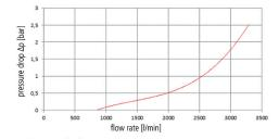
System pressure: 6 bar  $[\bar{u}]$  Flow value given at 0.5 bar pressure drop Flow depends on connection type and size of coupling and plug
