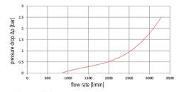
System pressure: 6 bar  $[\bar{u}]$  Flow value given at 0.5 bar pressure drop Flow depends on connection type and size of coupling and plug
