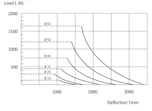
max. distance (SL) in mm - without mid section support / mid section mounting
