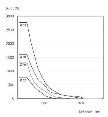
max. distance (SL) in mm - without mid section support / mid section mounting
